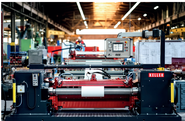
The film skiving machines enable the skiving of ultra-thin films from 20 µm with a thickness tolerance of ±3 µm, with skiving billet diameters of up to 800 mm and skiving billet lengths of up to 1600 mm © Keller HCW
